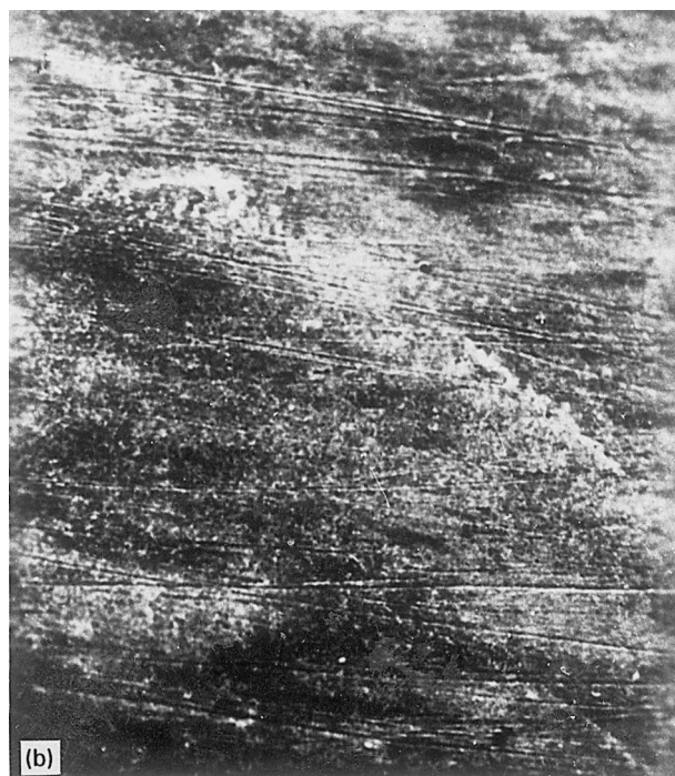
Figure 6 Scanning electron micrographs of the electrodeposited samples (X 25000): (a) 0.05 M, 30 \text{ mA cm}^{-2} , and (b) 0.2 M, 120 \text{ mA cm}^{-2} .
